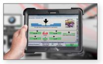
... or use SplashTop remote software for complete remote control of the aligner from your Apple or Android device.
